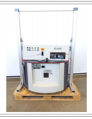
The FourC machine is for automatic measuring of gemstones which are not undercut during the rotation.
